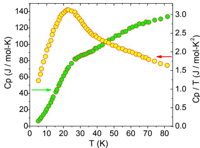
**Fig.2.** The temperature dependence of specific heat under zero magnetic field.
