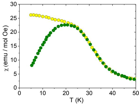
**Fig.1.** The temperature dependence of ZFC and FC susceptibility ( $\chi$ ) under a low field of 0.1 T.
